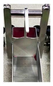
It is normal to see a small amount of leakage from the bottom of the gate (as pictured opposite).
